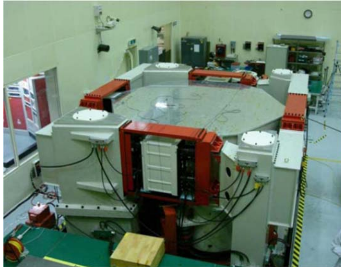
Figure 1 Current KARI Vertical Vibration System
